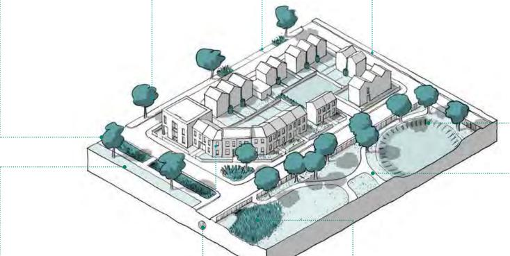
Swales: Shallow channels that provide attenuation while also channeling water to other features such as ponds.
