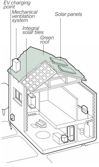
**Figure 90:** Cut-through diagram of an energy-efficient home and its features.
